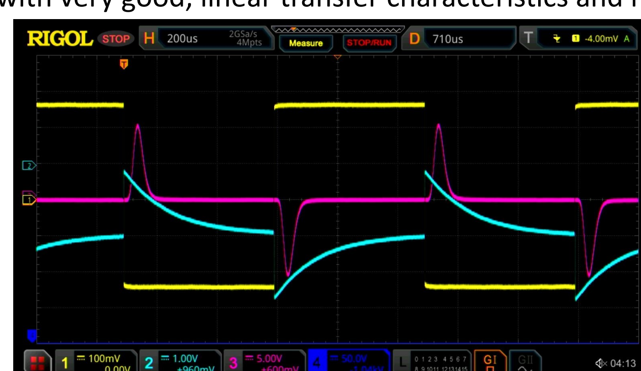
Figure 9-Output of first version of PCB (pink)
