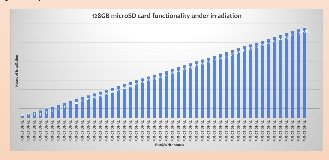
All microSD cards in batch 1 and batch 2 were still functional after exposure to the neutron source.
