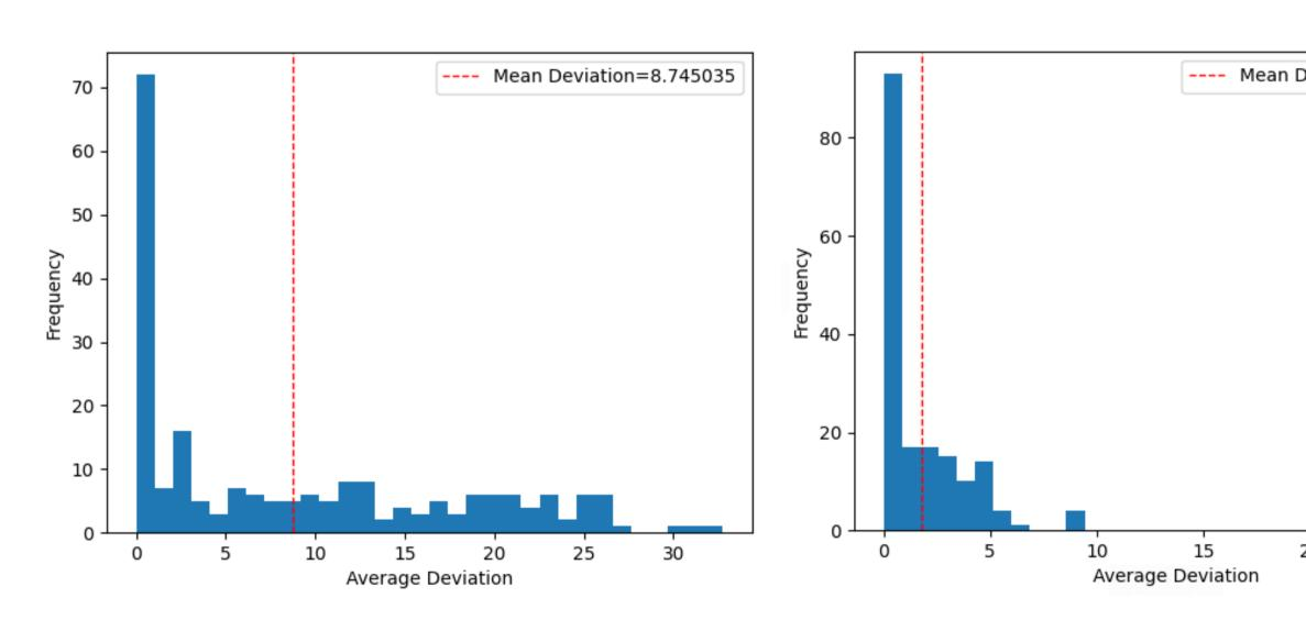
It was found that using a novel detector geometry increased the position sensitivity of the detector. This result can be seen in the deviation histograms for the cubic (left) and double French cut geometry (right) through the location of the mean. The novel geometry provides more information to the PSA from the additional reflections off the crystal faces.
