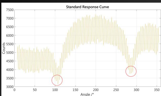
Figure 1 – A RadICAL SRC of <sup>137</sup>Cs, obtained during testing, clearly showing two minima at approximately 180° apart. Using two RadICAL detector SRC graphs, a source location and distance could be determined.
