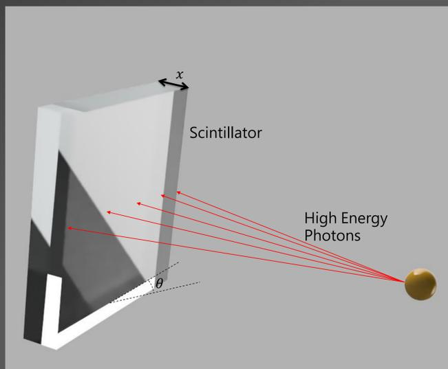
Figure 2 - Variation in the scintillator thickness and surface area as a function of angle. The maximum scintillator thickness occurs when the lowest surface area is presented to the radioactive source; this however, has an insignificant effect when compared to the effect of surface area.
