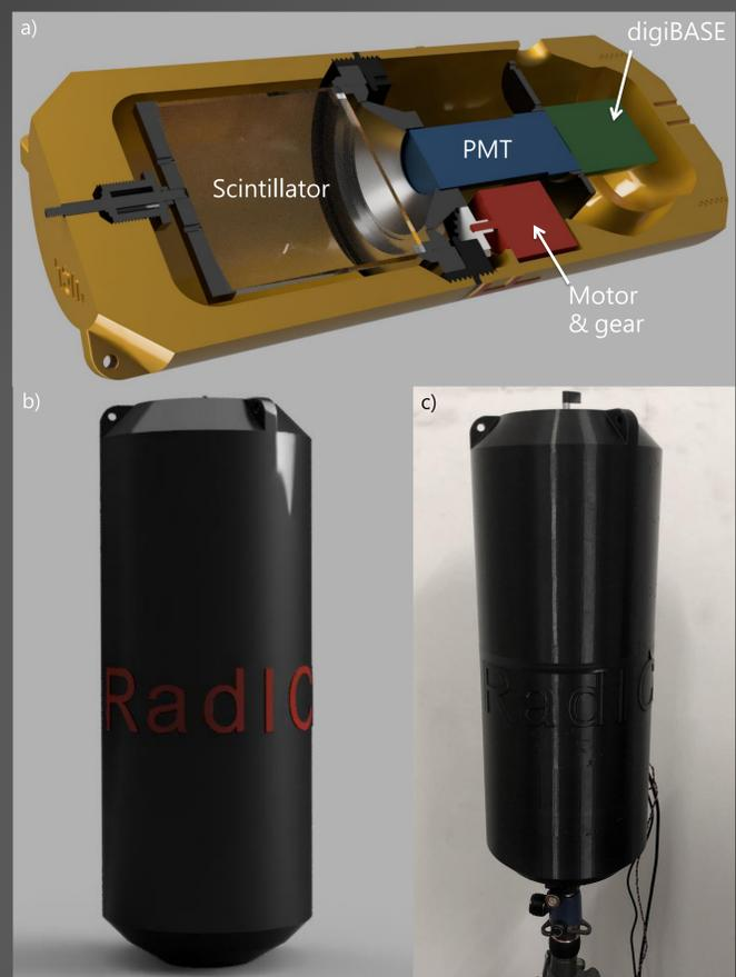
Figure 5 – a) A cross-section of RadICAL rendered in CAD software showing the basic elements of the RadICAL detector. b) A rendering of the outer housing of RadICAL. c) The functioning RadICAL detector prototype.
