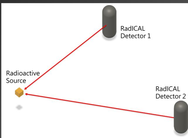
Figure 3 – Two or more RadICAL detectors could be used to determine the location of a radioactive source. This could be useful in the monitoring of ports and stations for homeland security.
