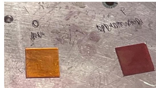
Figure 6: Top: Chemical compositions of the three isomer forms of carborane-NDI polymers (taken from [2]). Bottom: Picture of carborane-NDI films before top contacts were added via evaporation. Left: oCbT 2 -NDI. Right: pCbT 2 -NDI. A noticeable difference in colour may be seen in this picture between the two isomer forms.
