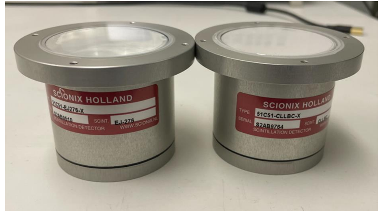
Figure 1: A picture of the plastic scintillator EJ-276 (left) and inorganic scintillator CLLBC (right).
