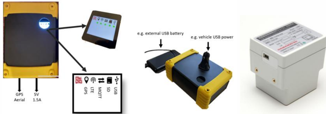
Figure 14: Example modular mapping units with 3.8x3.8x2.5 cm CsI(Tl) scintillator detectors (Hamamatsu).
