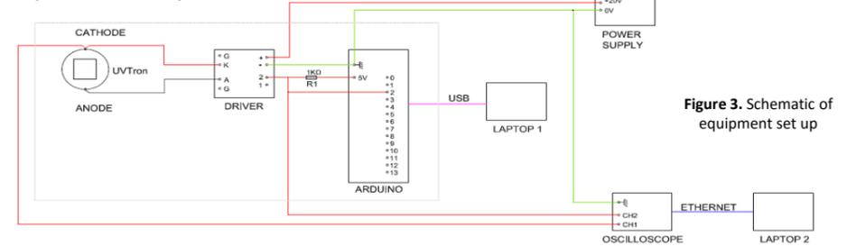
Figure 3. Schematic of equipment set up
