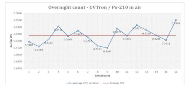
Figure 4. Average cps per hour – Po-210 source in air
