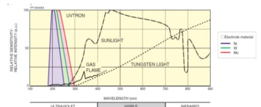
Figure 2. Spectral response of UVTron in comparison to sunlight, tungsten light and gas flame by electrode material.
