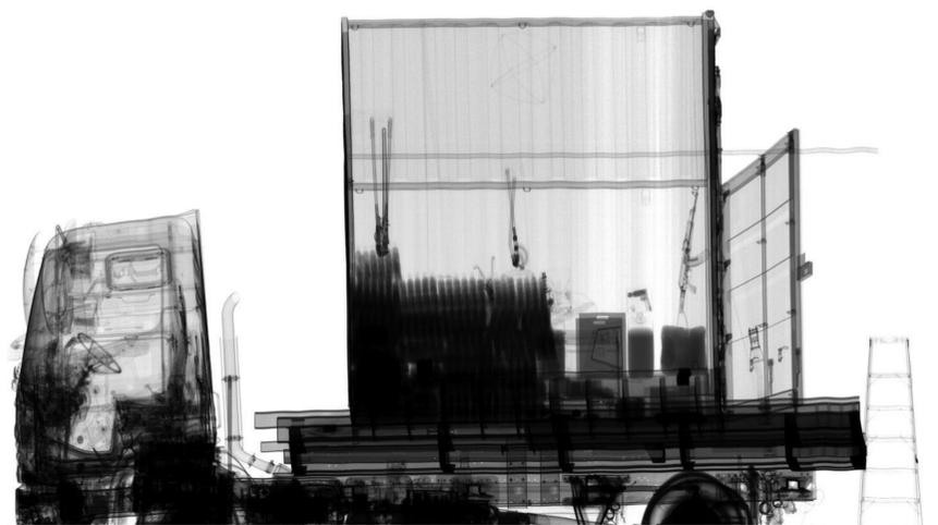
Figure 3. An X-ray scan of a truck[2]. Resolution is poor, and can't distinguish between some items inside the truck. It is hoped the use of TlBr crystals will increase the detector resolution.
