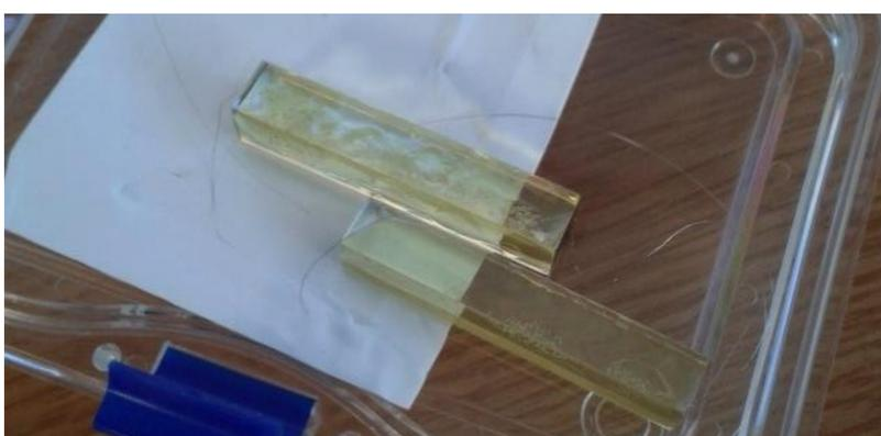
Figure 4. The two crystals supplied by CapeSym, with thin Palladium contacts visible.
