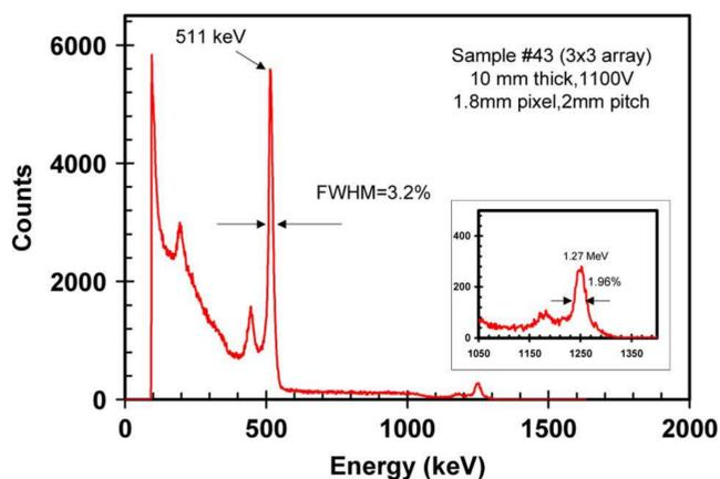
Figure 2. Room temperature spectra of 511 keV and 1.27 MeV gamma rays from one pixel of 10 mm thick TlBr detector.[1].
