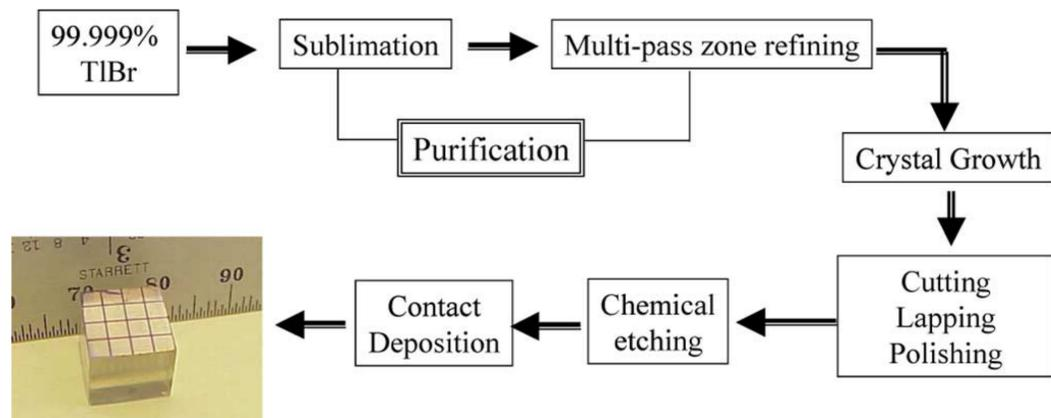
Figure 1. Diagram of steps taken to fabricate a TlBr Crystal [1].
