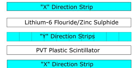
Figure 2: Diagram of the proposed detector design
